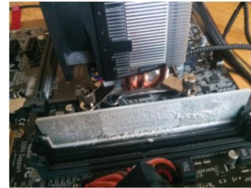
Figure 2: Cold Boot Attack on DDR4 DRAM. This photo shows the DRAM in one of our DDR4-based systems. The DRAM is filled with data scrambled by the memory interface of an Intel Skylake-based CPU. The memory has been cooled to -25^{\circ}C , and it will next be moved to a separate system where its contents will be descrambled.
